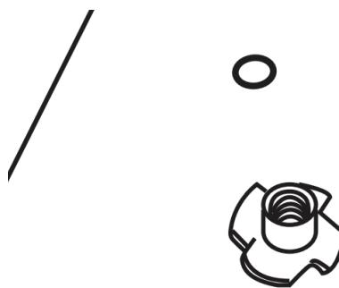
Flatten the Tee Nuts with a mallet or hammer
