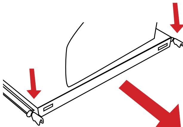
Mark the 8 drilling points through the slide fixing holes with a permanent marker
